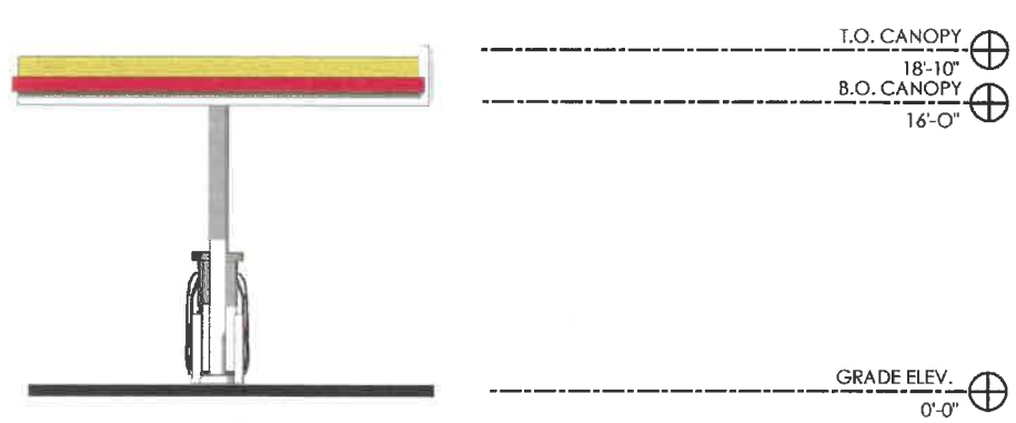
② North / South Canopy Elevation 1/4" = 1'-0"
